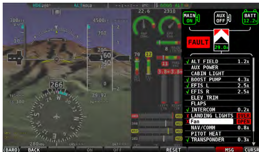
Figure 50 - VP-X Page with Fault
