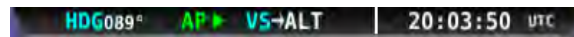
Figure 132–Pitch Axis Example: Vertical Speed mode, engaged and changing altitude to match altitude bug
