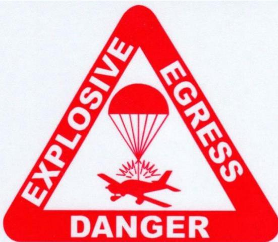
Rocket Deployed Parachute Egress Area
